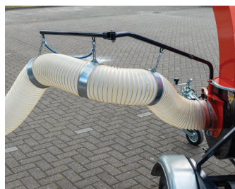
The suction hose with a 5 m radius is supported by a pivoting boom.
