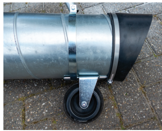
Castor wheel supports the weight while operating the suction hose.
