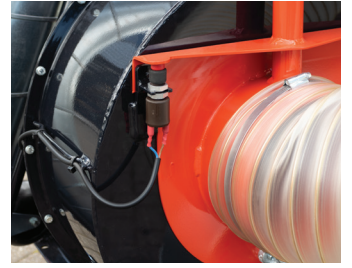
Safety sensor on fan housing shuts off engine during maintenance work.
