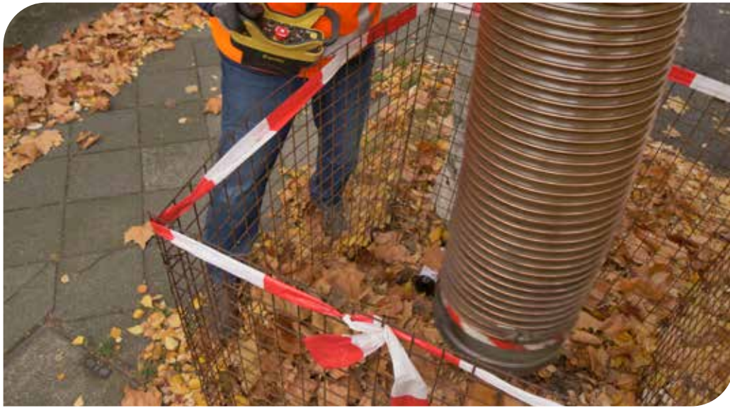
Automatic hose pendling moves the suction hose back and forth for better suction.
